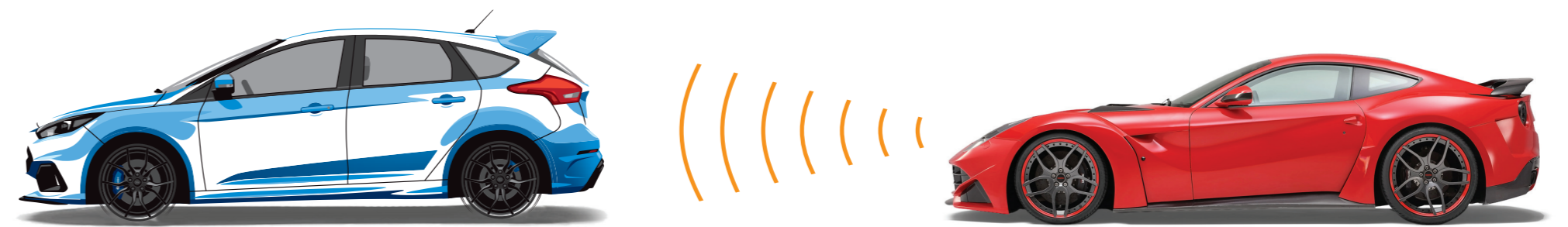
Figure 1: Adaptive Cruise Control based on FMCW Radar technology, operating in the 77GHz band
