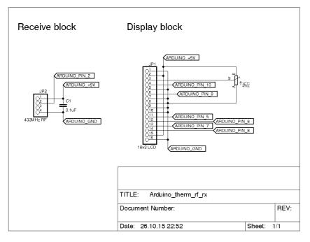
Please note that the receiver is an Arduino Mega, and it is not in the schematic. Follow the labels on the schematic to connect to the Arduino Mega.
